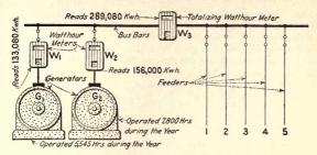
Fig. 52.—Examples in determining average loads.
